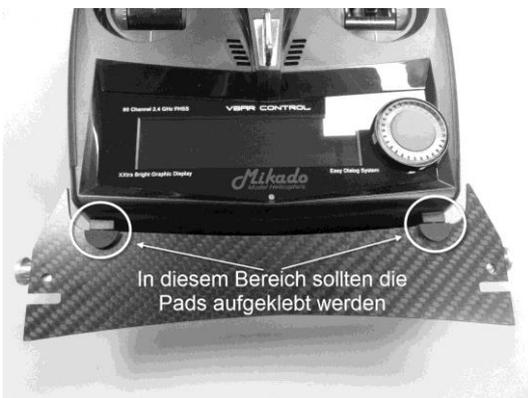
III. 5 Pads should be applied (glued) in this area
