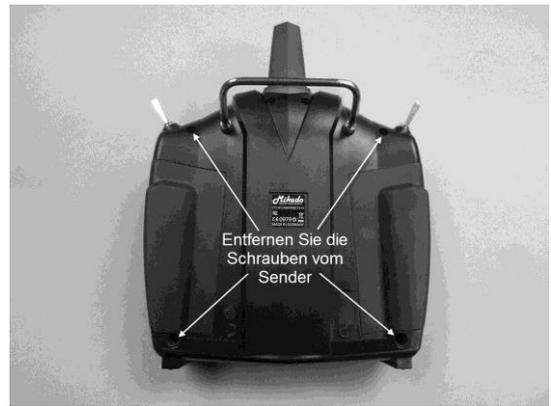
III. 2 Remove the screws from the control
