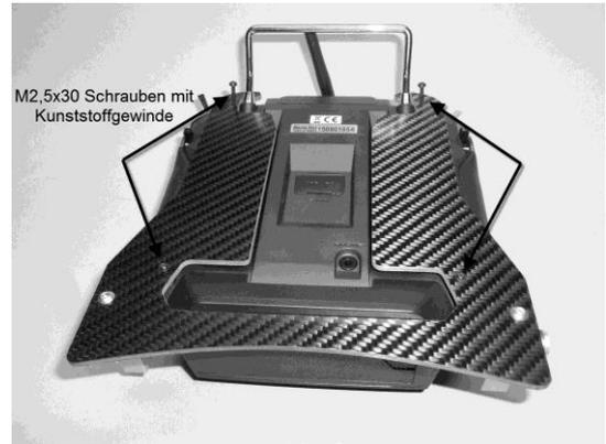
III. 2 M2,5x30 screws with synthetic thread
