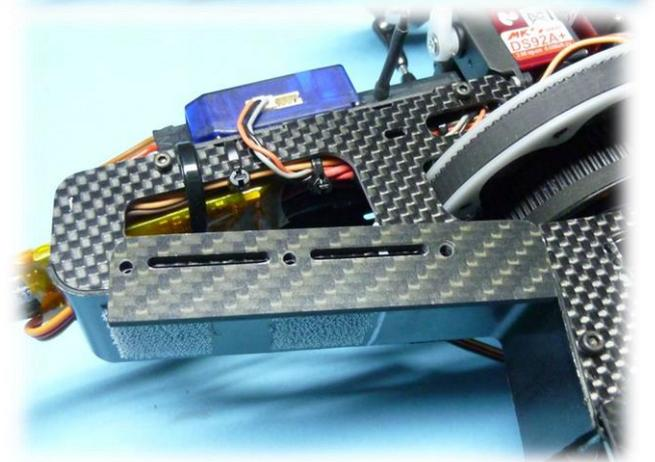
Then position the bearing plates onto the guide plates and fix, at the moment only slightly, with the supplied screws.
